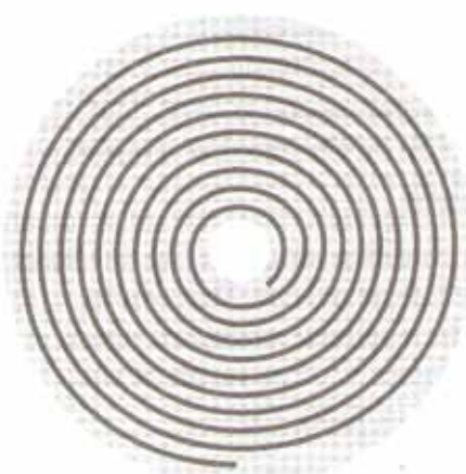
Figure 1.6 The pits and the lands are placed along a spiral on the surface of the disk.
