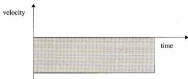
Figure 1.9 The velocity-time graph for uniform motion towards the left.
