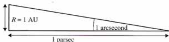
Figure E3.2 The definition of a parsec. A parsec is that distance at which 1 AU subtends an angle of 1 arcsecond.
