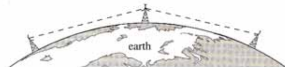
Figure F4.7 A microwave link.
