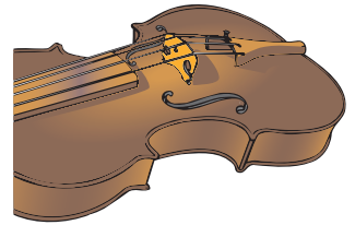
Fig. 9.2.14 A violin's bridge transfers energy from its vibrating strings to its belly. The belly moves in and out, emitting sound. Some of this sound leaves the violin through the S-holes in its body.
