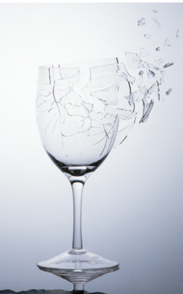
Fig. 9.2.6 Resonant energy transfer makes it possible for sound to shatter a crystal wineglass. When the sound pushes on the glass rhythmically, the sound slowly transfers energy to the glass, until it finally shatters. Because the sound must be extremely loud and at exactly the resonant frequency of the glass, only the most extraordinary opera singers can break a crystal wineglass.
