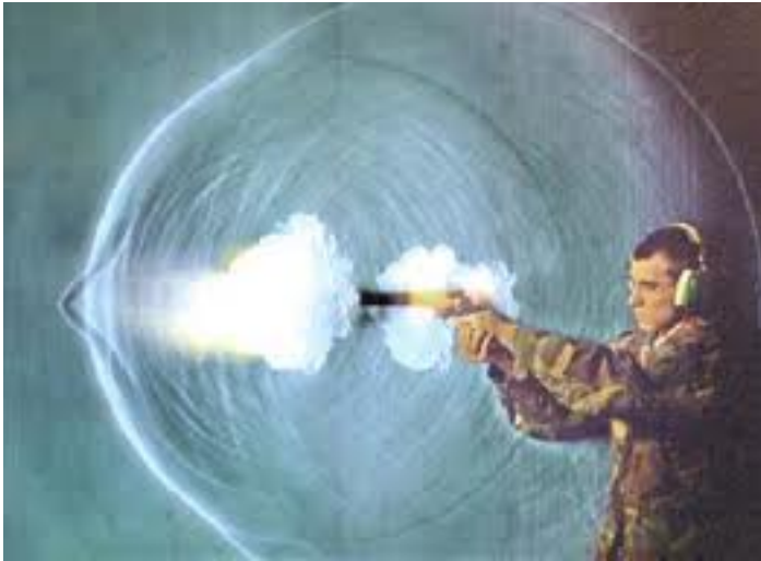
Record of shock waves produced by bullets
